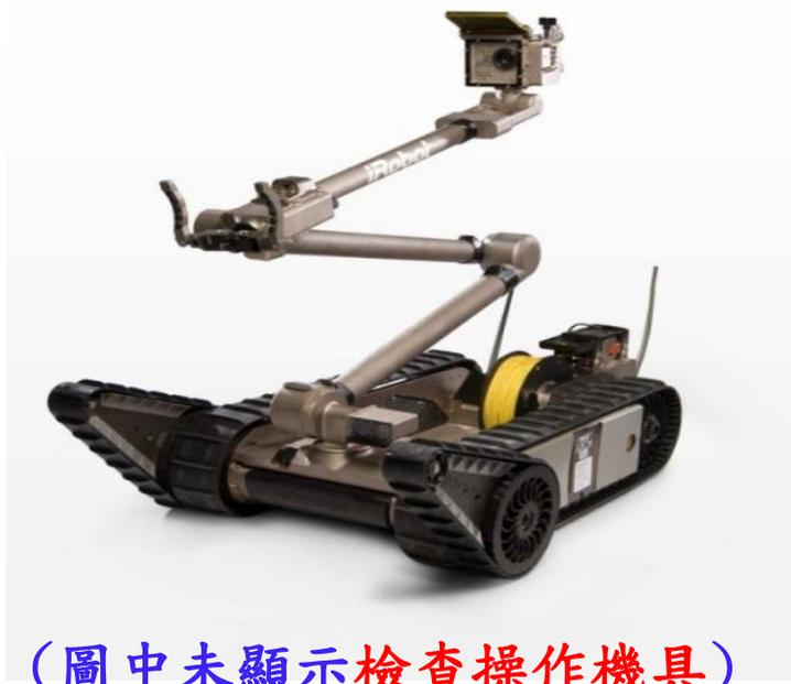
**Use of Robotics and Remote Monitoring Equipment for Reducing Dose and Risk Associated with Radiological Work at Ontario Power Generation**
