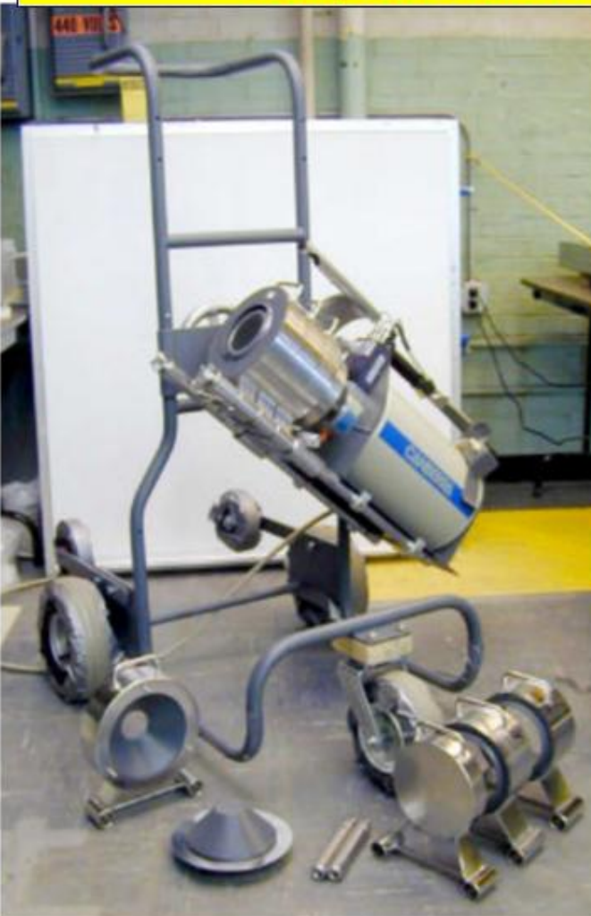
ISOCS cart with detector, cryostat and modular shield system
