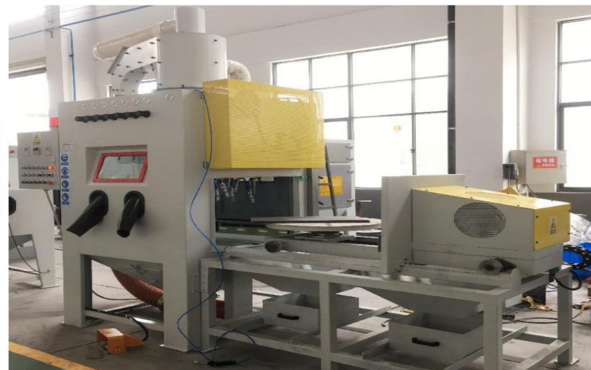
Sandblasting Turntable and Track System
